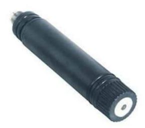
Universal sensor body, PPS construction. Models available for pH, ORP, low ionic strength solutions, and HF-resistant electrodes for solutions that should not exceed 1% hydrofluoric acid. Order pH electrode adapter at left to connect the new ERP-series electrodes to olderstyle cartridge electrode cap cable installations.
