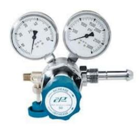
Ideal for corrosive or noncorrosive gas applications. Designed and constructed for diffusion resistance and easy cleanup. Only brass, stainless steel (SS) , PTFE, and Kel-F® contact the operating media. Metal diaphragm, packless valves, and high-purity seals minimize or eliminate outgoing and inboard diffusion. Supplied with SS screen filter (25  $\mu m)$ ; and brass body, bonnet, and gauges. Two-Stage High-Purity Regulators let you precisely regulate working pressure.
