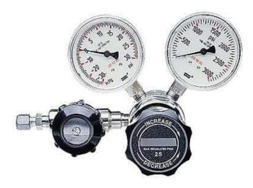
Model 03274-10 is a single-stage unit specifically designed for gases that attack brass or copper-bearing alloys. When used with low-vapor-pressure liquefied gases, no inlet gauge is needed. Rubber-supported PTFE diaphragm, KEL-F seat, aluminum-alloy body and bonnet, SS delivery gauge, and 10 mm sintered SS filter.
